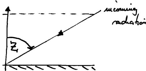
$$F_{sw} = F_{sw}^{\circ} \cos Z \quad \text{where } F_{sw}^{\circ} = S \left( \frac{d_m}{d} \right)^2$$
