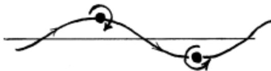
Figure 14.1 Showing how a parcel of fluid moved northward in a standing wave, conserving its potential vorticity, \zeta + f , develops negative (anticyclonic) spin, \zeta , which affects fluid to the east and west, reinforcing the north-south motion of the
